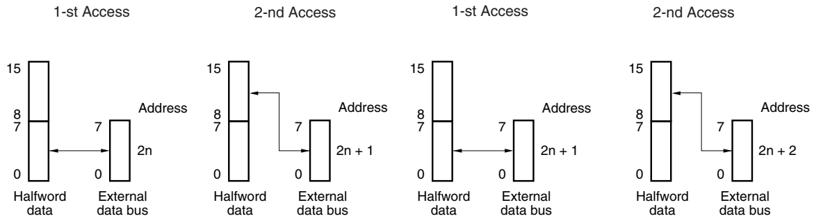
Figure 7-23 Left: Access to even address (2n) Right: Access to odd address (2n + 1)
