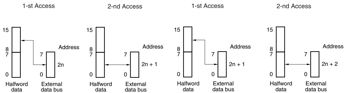
Figure 7-24 Left: Access to even address (2n) Right: Access to odd address (2n + 1)
