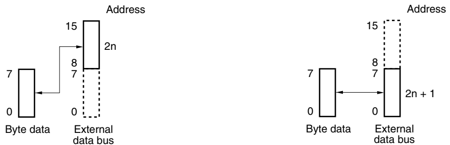
Figure 7-34 Left: Access to even address ( 2n ) Right: Access to odd address ( 2n + 1 )
