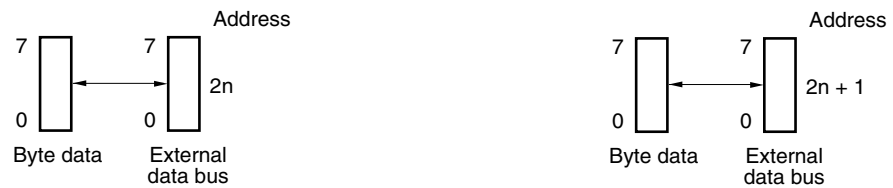
Figure 7-22 Left: Access to even address ( 2n ) Right: Access to odd address ( 2n + 1 )
